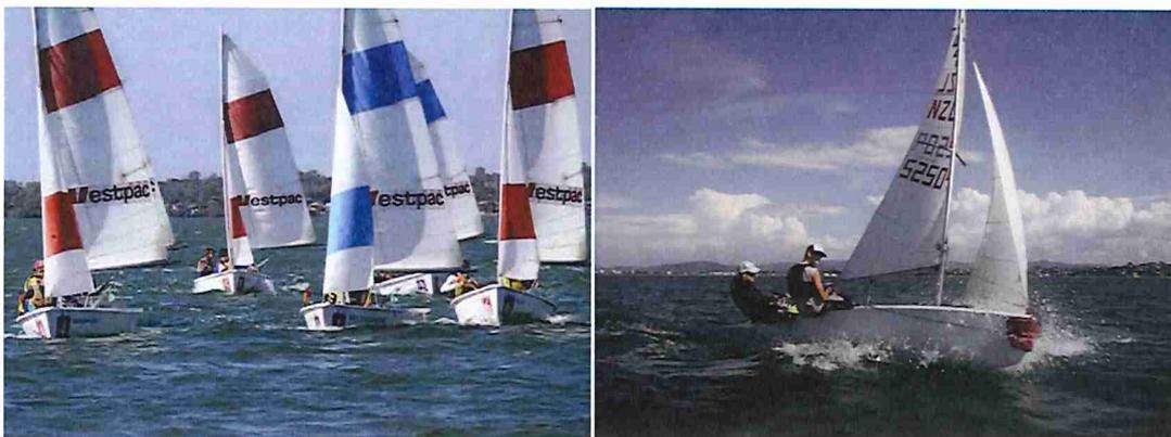
Our teams racing program is run in international 420 dinghies, specially modified for teams racing (above right). They are a lightweight and powerful fibreglass dinghy, 4.2 meters long and designed for paired sailing with a helm and crew weight between 110-145kg.
